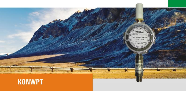
The wireless pressure transmitter KONWPT is a part of the wireless pipeline pressure monitoring system. The KONWPT is a battery powered autonomous unit for pipeline pressure measurement. Measuring data is sent over a 2,4 GHz wireless radio link to the Access Point. APs collect measured data from KONWPTs, and send it through to the Modbus Gateway to the pipeline monitoring center.
