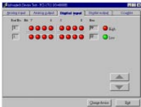
Fig. 2-14 Digital Input tab on the Device Test dialog box
