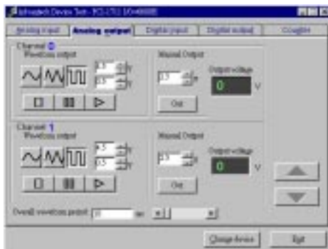
Fig. 2-13 Analog Output tab on the Device Test dialog box
