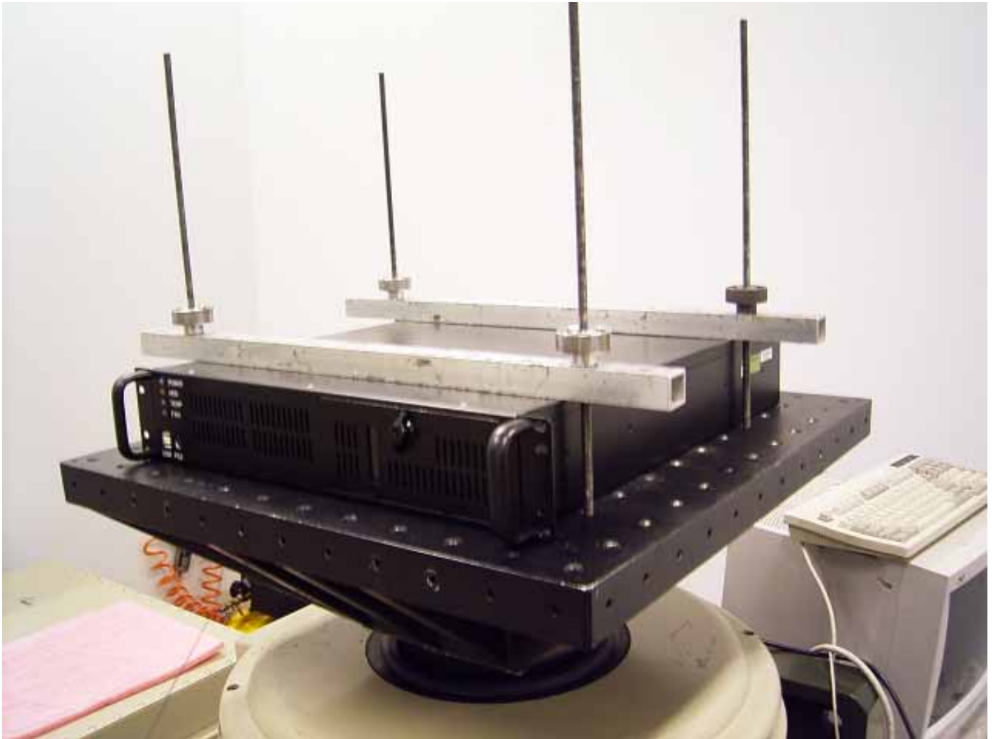
ACP-2320MB Sine vibration test Z axis
