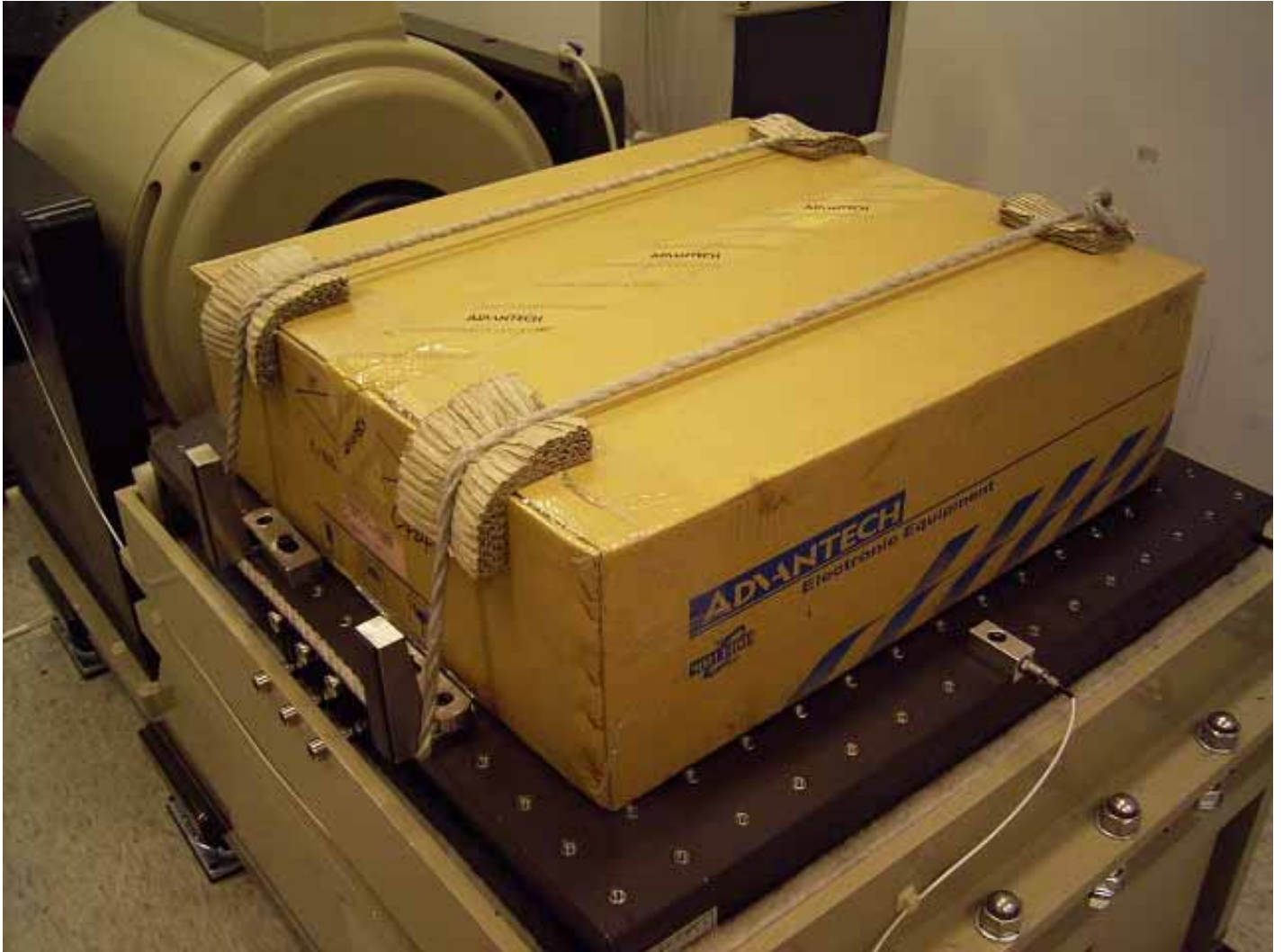
ACP-2320MB package vibration test X axis
