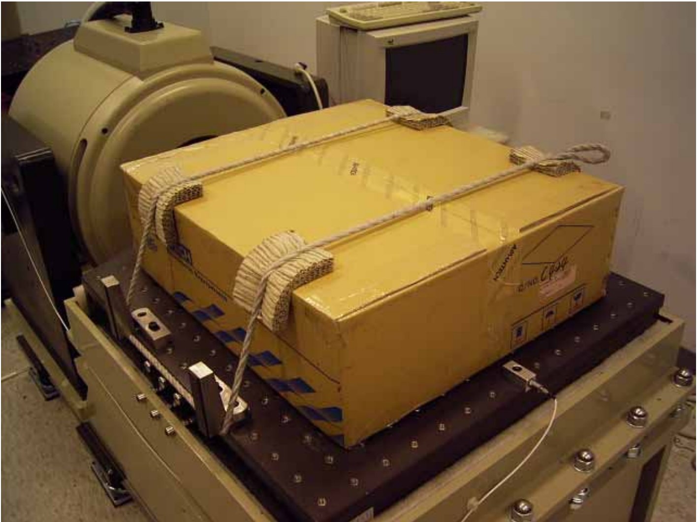
ACP-2320MB package vibration test Y axis
