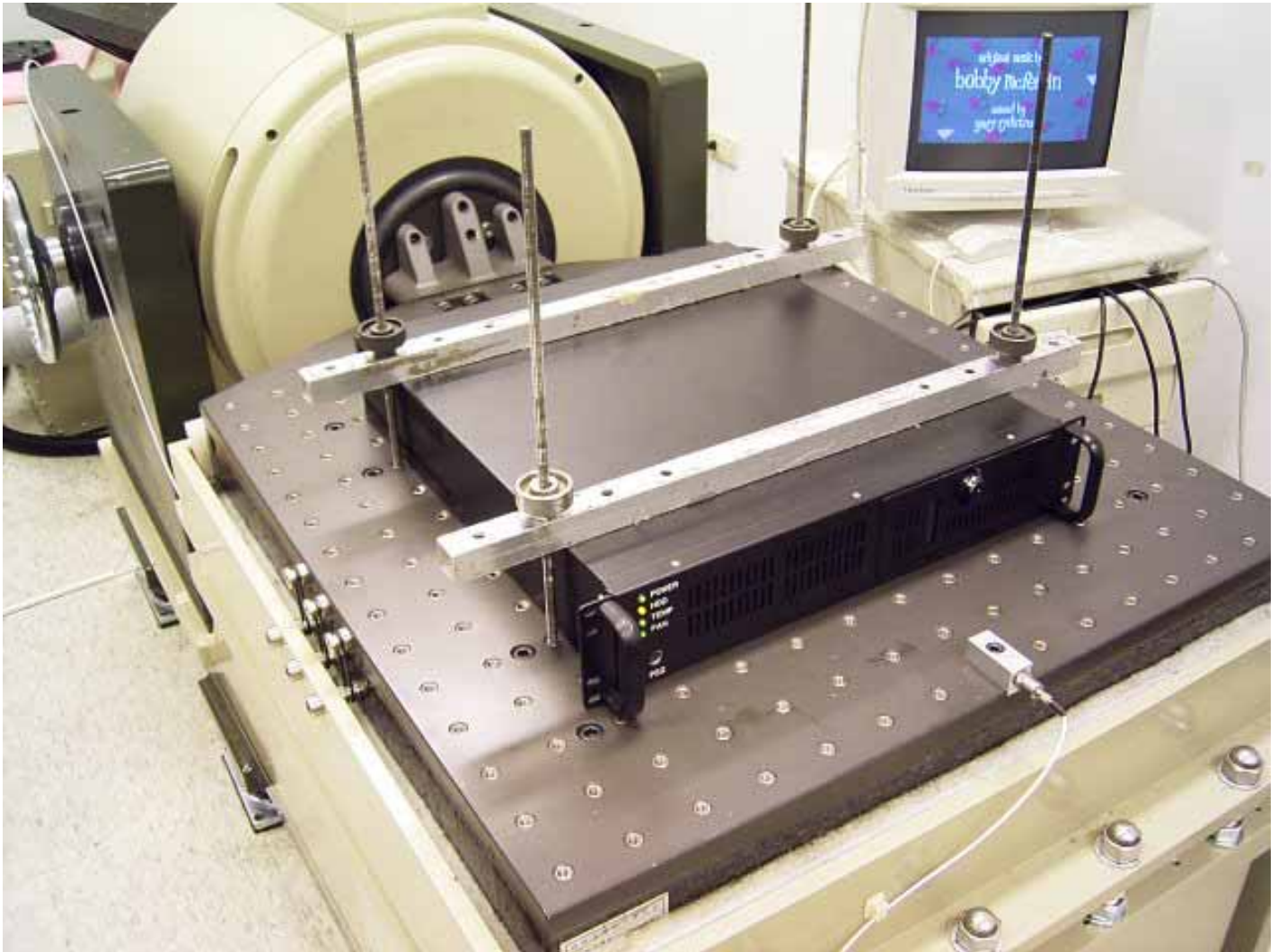
ACP-2320MB Random vibration test Y axis
