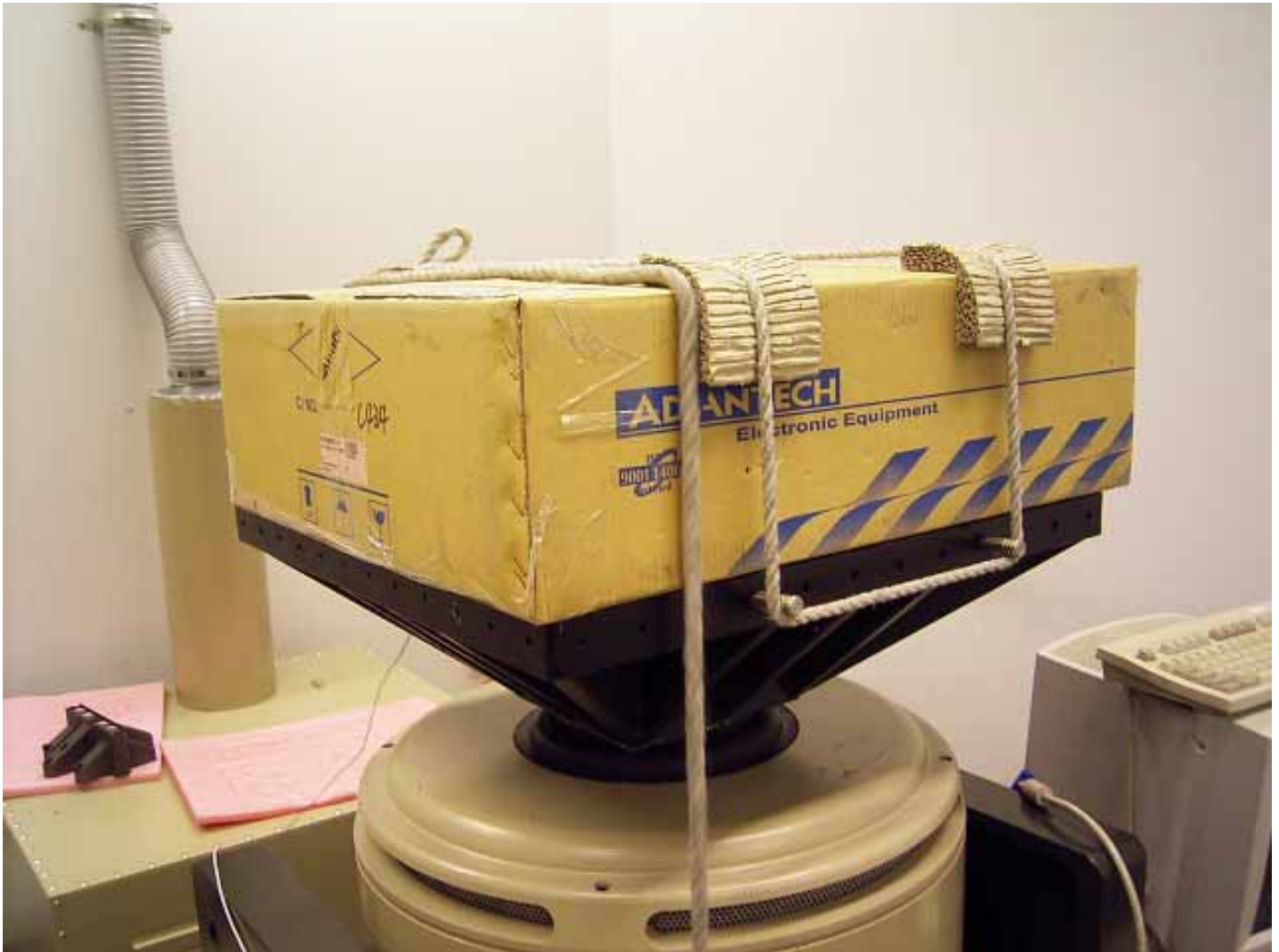
ACP-2320MB package vibration test Z axis
