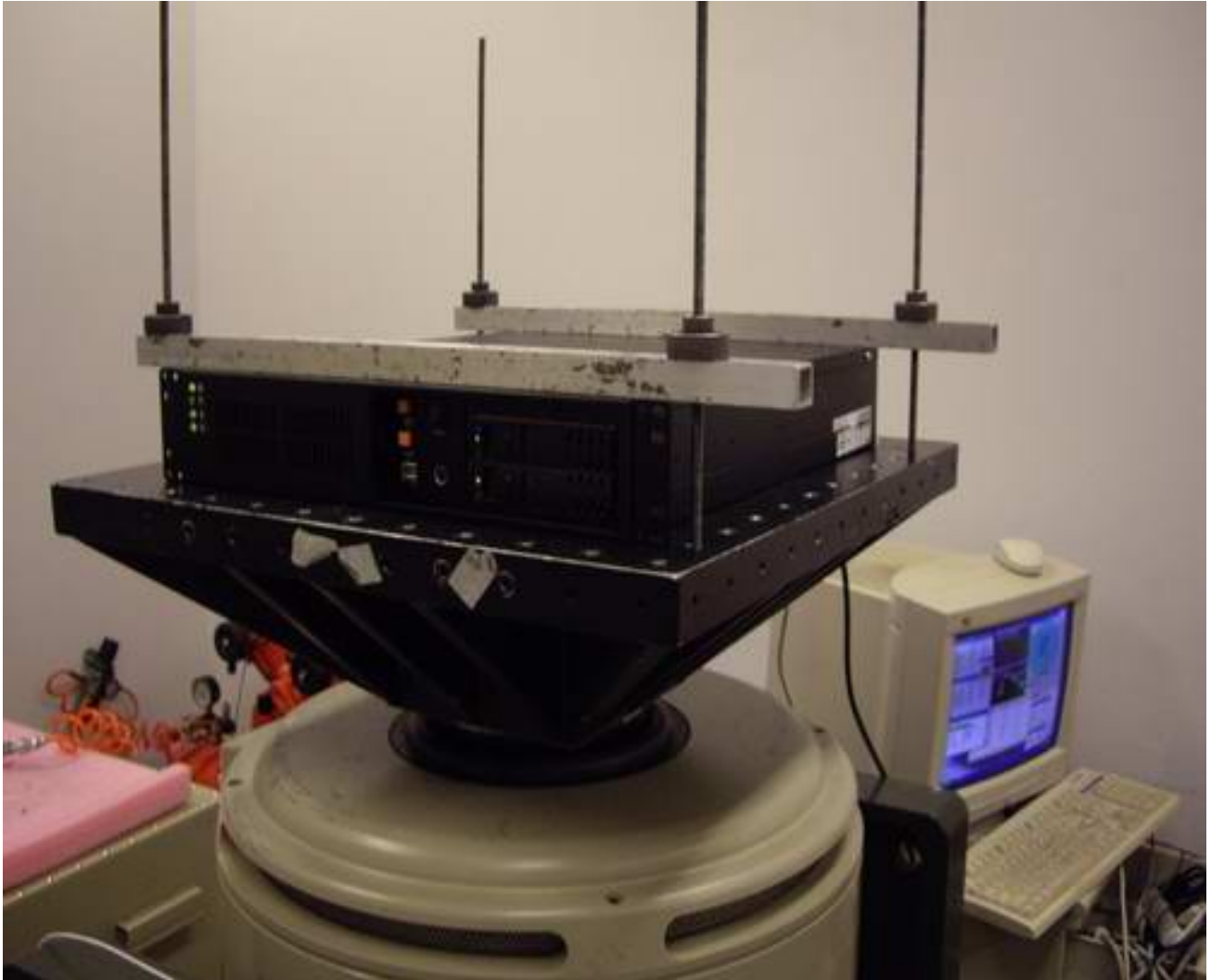
ACP-2320 random vibration test for Z-axis
