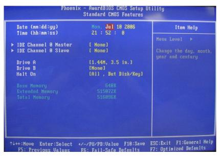
At the bottom of the menu are the control keys for use on this menu. If you need any help in each item field, you can press the <F1> key. It will display the relevant information to help you. The memory display at the lower right-hand side of the menu is read-only. It will adjust automatically according to the memory changed. The following pages describe each item of this menu.
