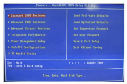
The section below the setup items of the Main Menu displays the control keys for this menu. Another section located at the bottom of the Main Menu, just below the control keys section, displays information on the currently highlighted item in the list.
