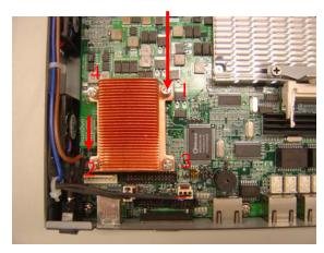
Fix the CPU heatsink on the socket
