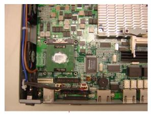
Insert the CPU into the socket
