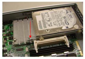
Figure 2-6: Install HDD
