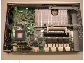
Unlock the socket of CPU as the symbol accordingly
