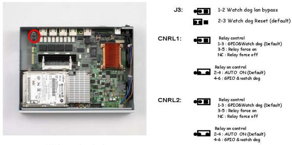
Figure 2-9: LAN Bypass function jumps
