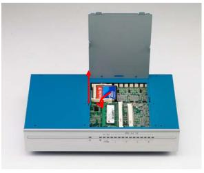
Figure 2-5: Install RAM module
