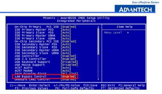
Figure 2-10: Setting LAN Bypass function from BIOS
