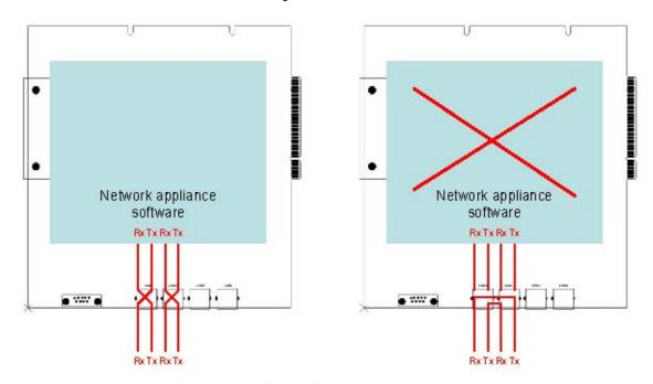
Figure 2-8: The illustration of LAN Bypass function
